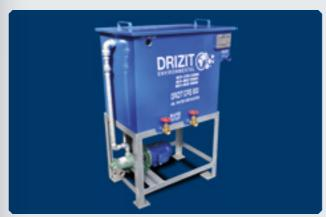
Designed for efficient oil removal in low flow between 300L per hour – 2000L per hour using a patented polypropylene coalescer. They require no supervision, minimal maintenance and once installed are fully automatic. Ideal for process effluent, wash bays, compressor blow-down and tramp oil removal.
